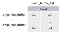
The image below is an example of a buffer\_list with 3 x flat\_buffer's pointing to 3 different physical memory addresses where the buffers (data) reside.
